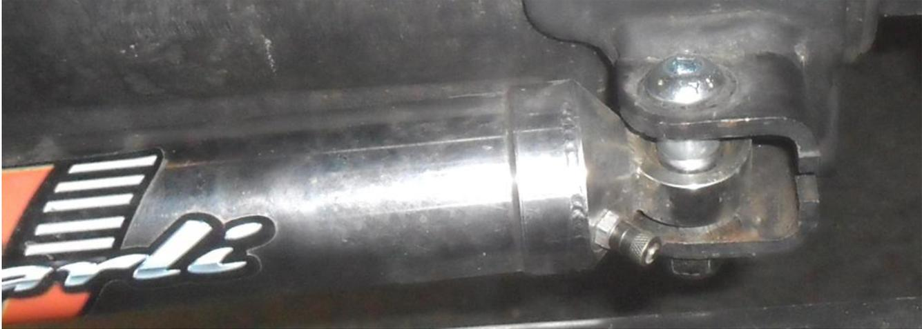
8. Adjust the stabilizer to desired pressure within operating range of 70-200psi as stated in "Special Notes"
