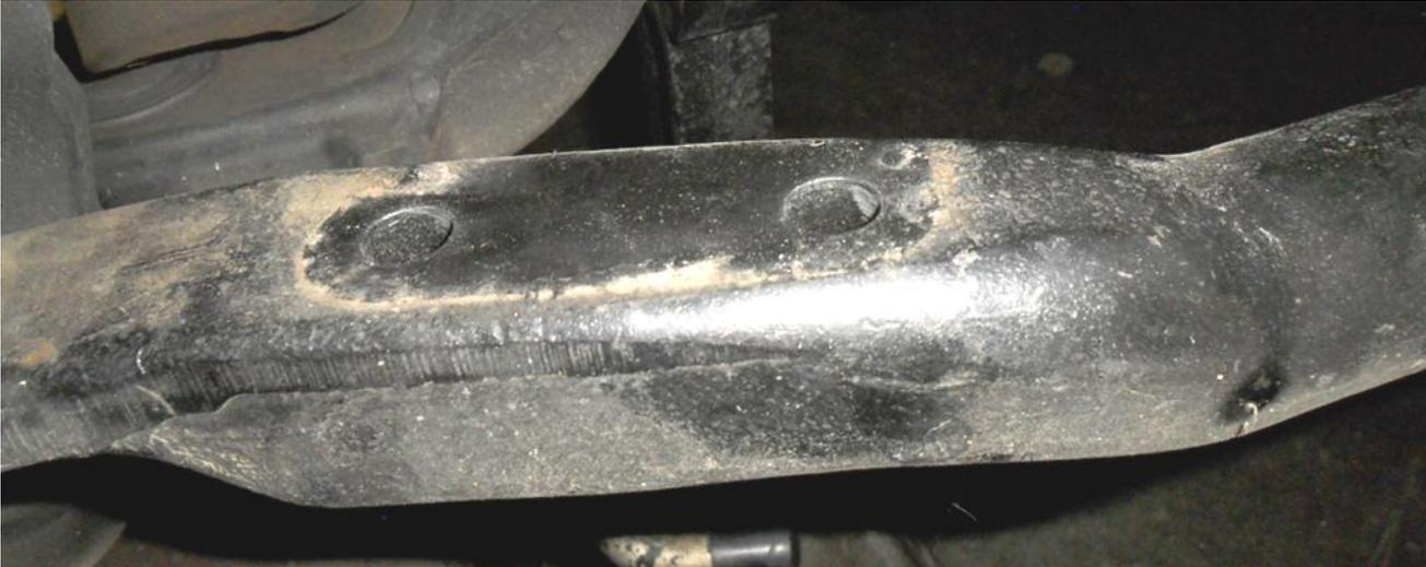
3. Install provided Carli Stabilizer Bracket onto tie-rod (where the factory bracket was removed). Bolts hand tight for now.
